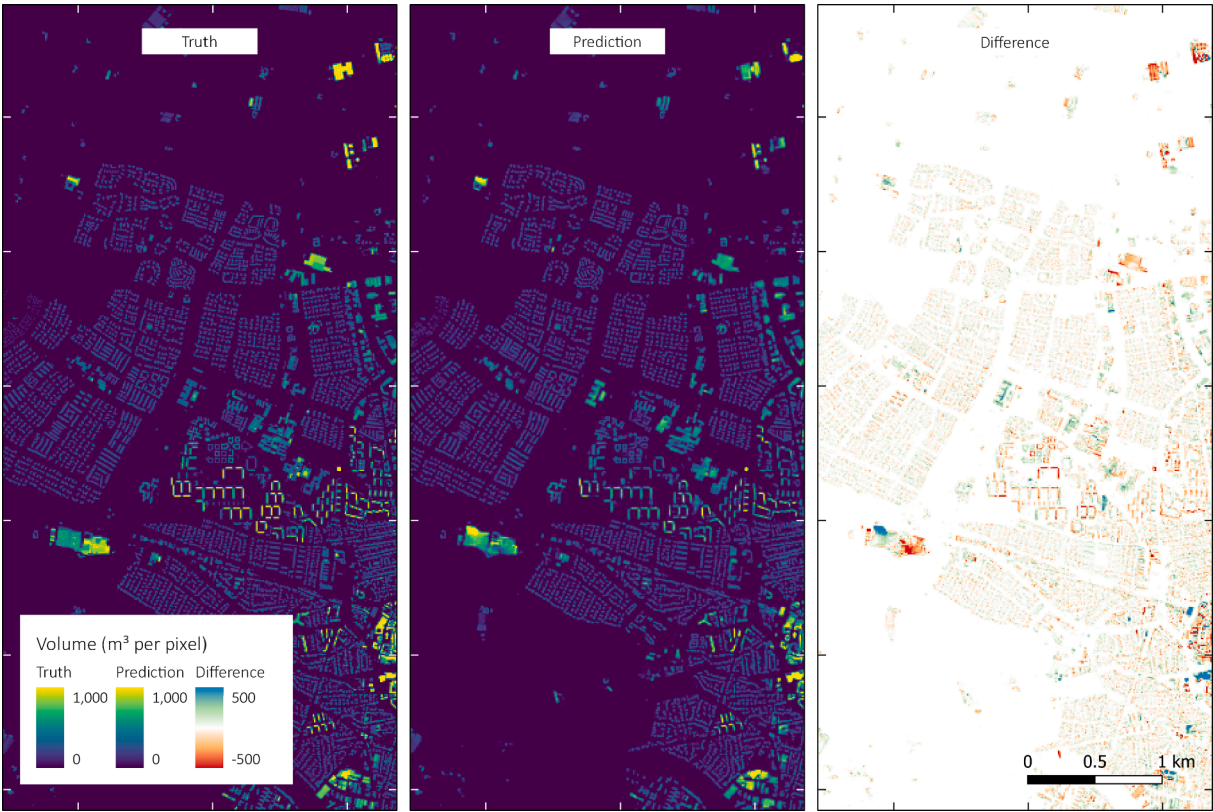
Fig. 13. Comparison between prediction and truth for building volume.
