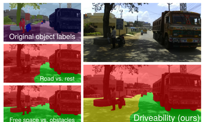
Fig. 2. Example of a pixel-annotated outdoor scene from the IDD dataset [20]. We map the original object classes to driveability levels.
