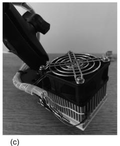
Figure 1. Quantitative thermal stimulating device (VICS, Tokyo) (a) consisting of a controller box (b) and a probe (c). (a) A broader overview of the device, with (b) representing the controller power unit and (c) representing the probe. Electric current to the Peltier element is controlled by a microcomputer in a controller box (b) connected to a PC via serial communication. Probe of the quantitative thermal stimulating device (c).
