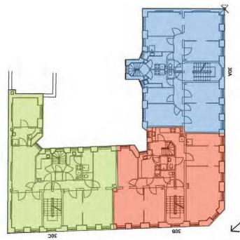
Figure 2. Horizontal cross section showing the apartment layout of the building. Blue is stairwell A, red is stairwell B and green is stairwell C.
