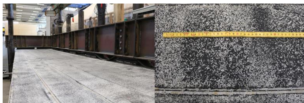
Figure 8. Contrast pattern on slab surface.
