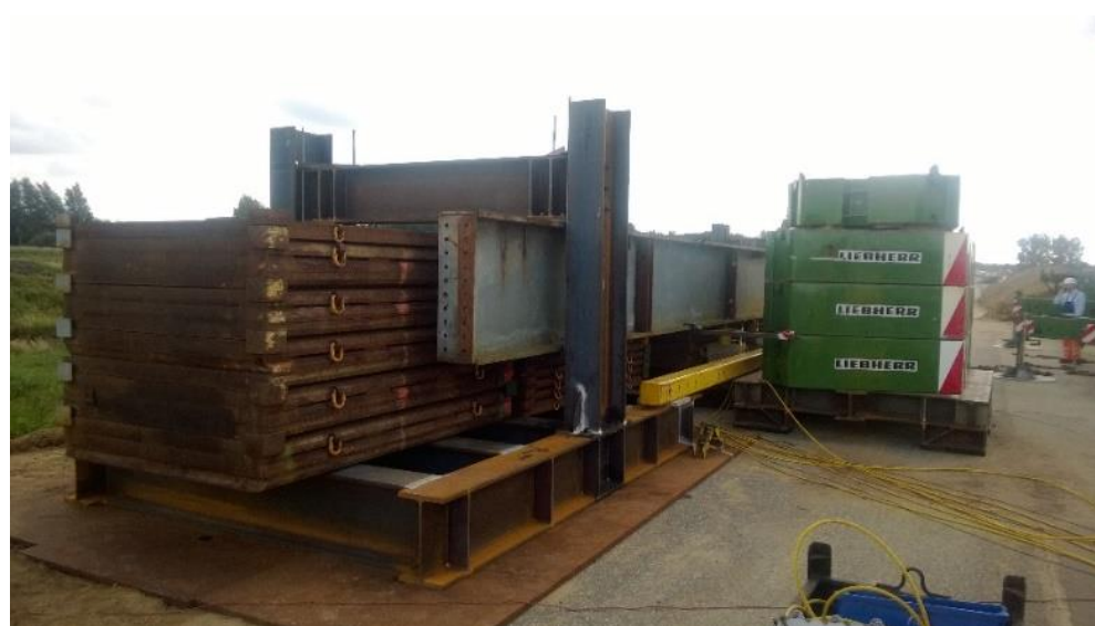
Figure 2. Applied classification loads used for the in situ tests. Standard vehicle A adjacent to standard vehicle B.
