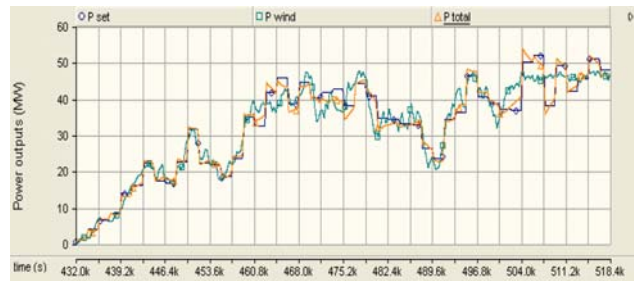
Fig 2. Active power output from fixed speed turbine based wind farm (light blue trace – active power without storage, dark blue trace – ½ hour active power set point based on wind prediction, orange trace – active power with storage)[32]
