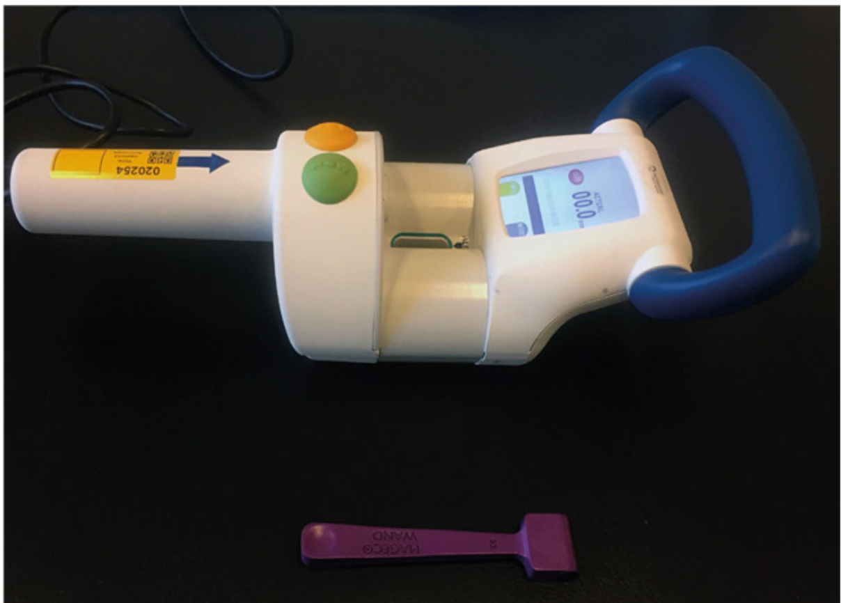
FIGURE 1 The external actuator (to be placed on the skin of the patients) with display on 0.0 and the magnet finder (lilac colour).
