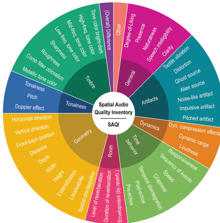
Fig. 5.5: SAQI wheel for the evaluation of virtual acoustic environments, structured into informal categories (inner ring) and attributes (outer ring). For definitions and sound examples refer to depositonce.tu-berlin.de/handle/11303/157.2 (CC-BY, Fabian Brinkmann).
