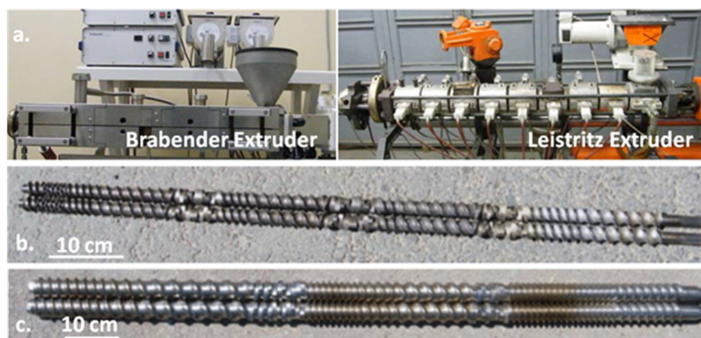
Figure 1. The lab-scale extruders used in the tests (a); screw profiles of the Brabender (b) and Leistritz (c) extruders.
