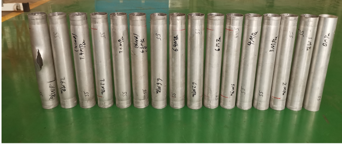
Figure. 7.1. Hydro-bulged tubular samples at multiple pressure levels.
