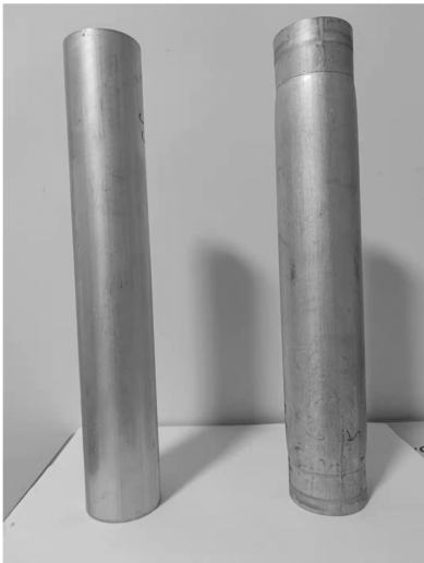
Fig. 6. Illustration of the initial and deformed 5049-O aluminium tubes in hydraulic bulge test with fixed end-condition.
