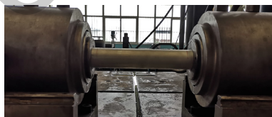
Fig. 8 Locking system for ends of tubular specimens on machine.
