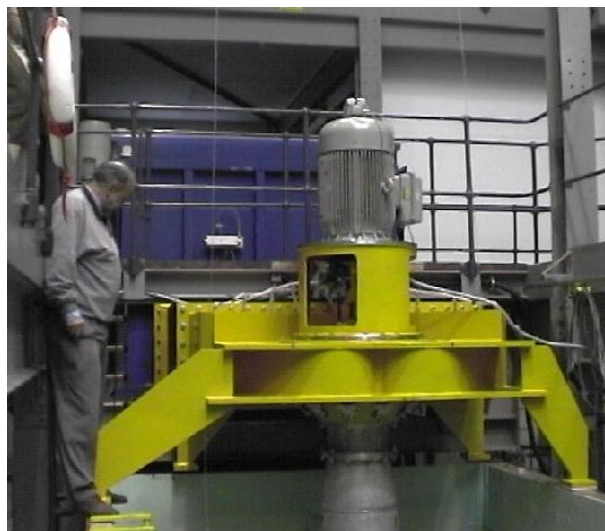
Figures 3 and 4: The Wave Dragon on/off turbine in full scale with cylinder gate and the existing test turbine in scale 1:3,5 at the test stand at Technical University Munich.
