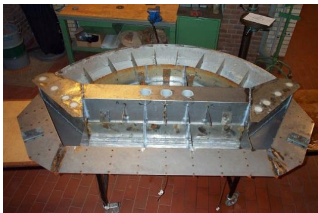
Figure 8: Photo of the Wave Dragon reservoir part. Taken from below during initial ballasting.
