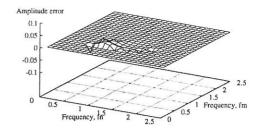
Figure 1: Theoretical long wave transfer function,  $F_{1,nm}$ , for piston type wave generator (left) and corresponding relative amplitude error,  $\epsilon_{nm}$ , when using the method presented in the paper (right).
