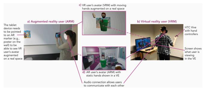
Fig. 3. Telexistence system used by ARM (a) and VRM (b) users. The users are presented to each other as virtual avatars: VRM avatar (c) with moving hands augmented on a real environment and ARM avatar (d) with static hands shown in a virtual environment.
