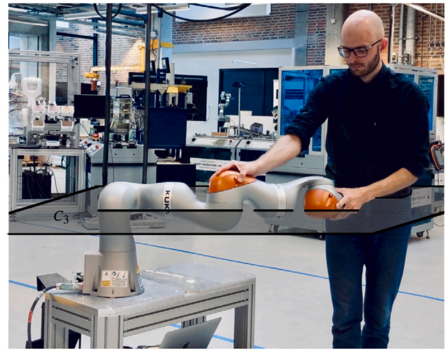
Fig. 5. Visualization of the enforcement of virtual workspace constraints while the manipulator is in a compliant state [62].
