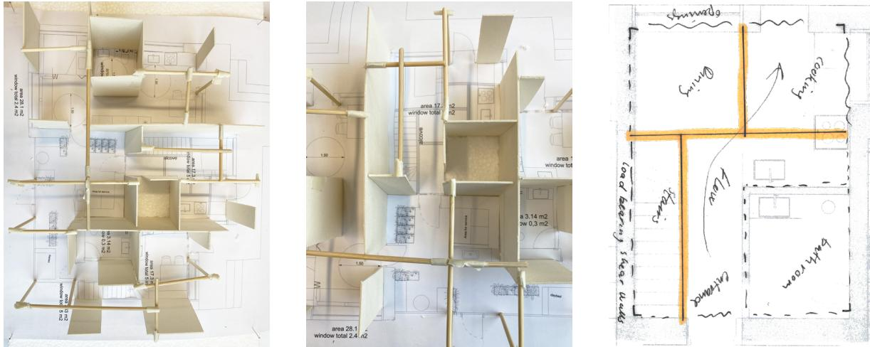
Ill. 149) Reciprocal system combined with columns and shear walls.
