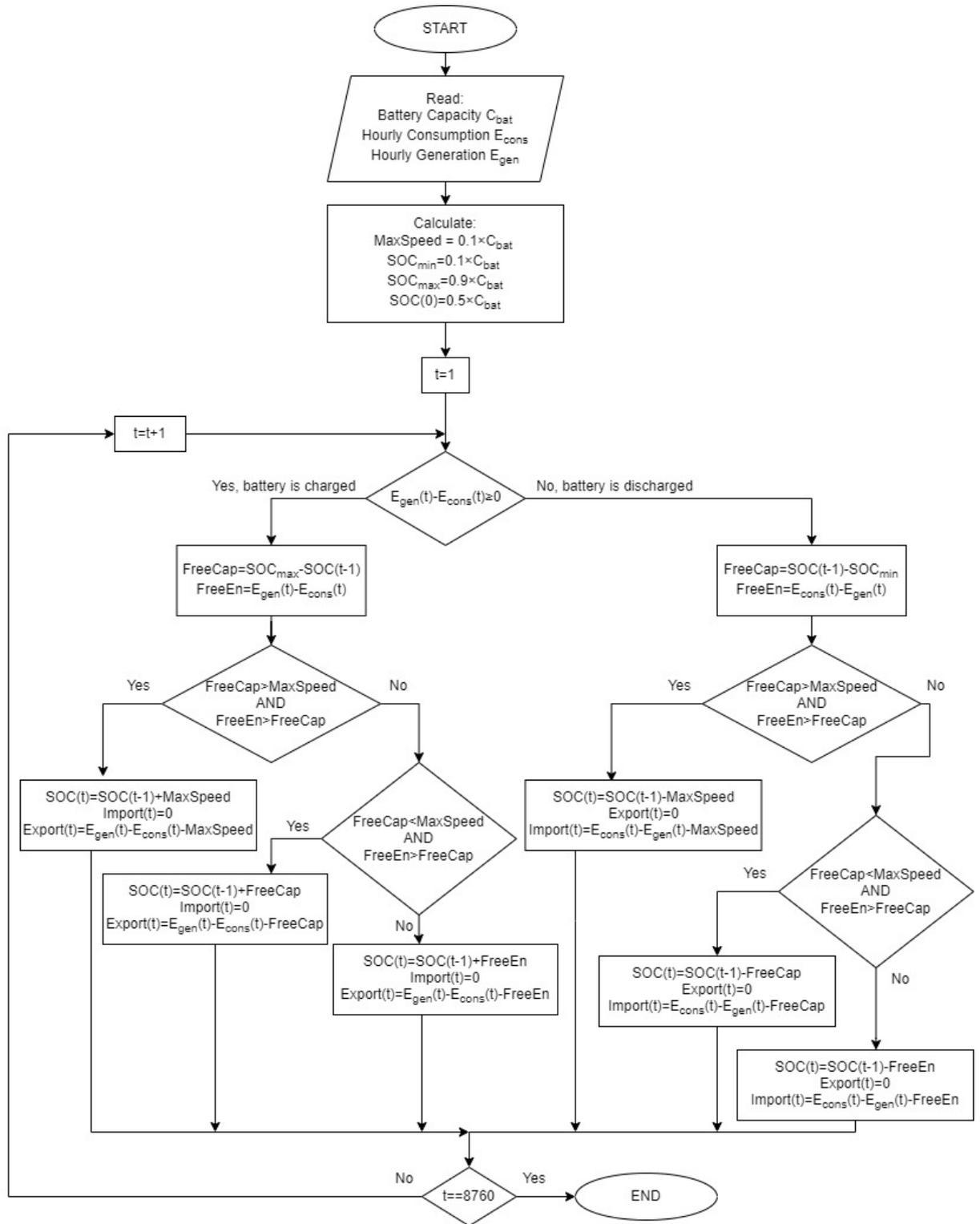
Figure 4.7: Flowchart showing the (dis)charging algorithm
