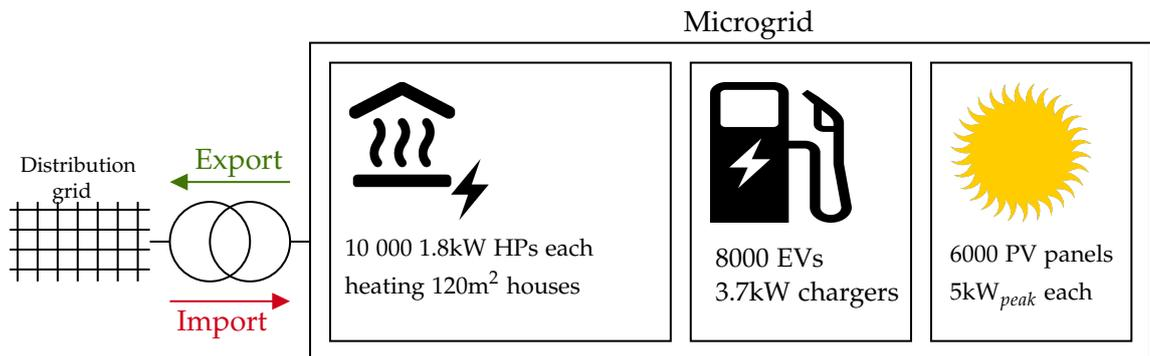
Figure 4.2: Tested microgrid and its components
