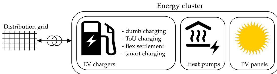
**Figure 4.1:** Energy cluster and its components
