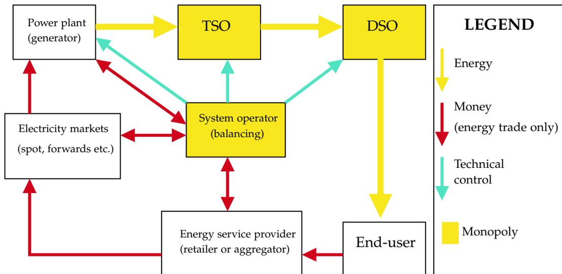
**Figure 2.1:** Simplified diagram showing different roles in a liberalised electricity market
