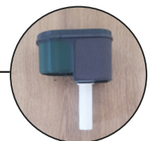
III. 70 The box fits in the ventilation, but it was too short to close to the fan.
