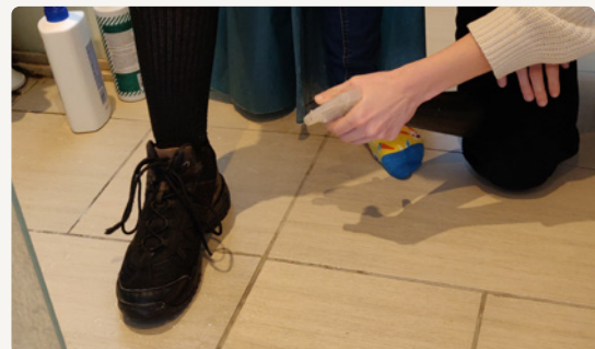
ILL. 11 The hiking boot was sprayed with water, in order to simulate the external conditions and control the amount of added water
