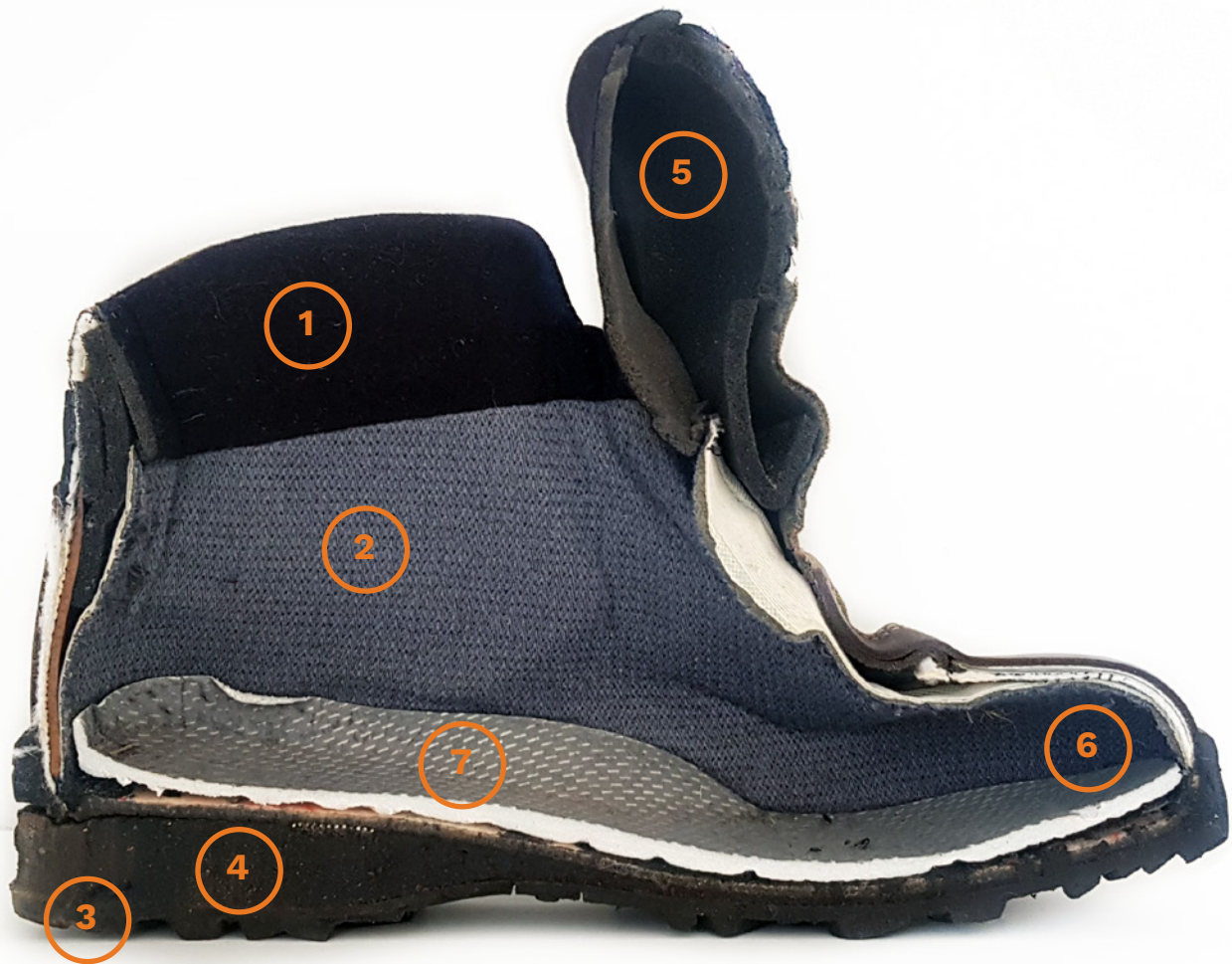
III. 26 A hiking boot cut in half shows the hidden construction and component of the boot.
