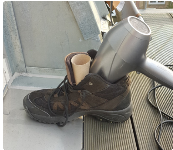
△ ILL. 39 The picture above is a hair dryer drying a hiking boot from the principal test (p. 29). Even though it dried the boot in 1h20min it need 3.214Ax-1h20x1000 = 4499.6mAh .
