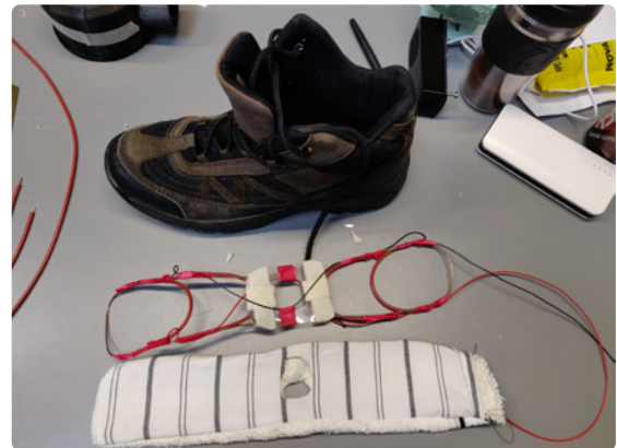
△ ILL. 40 The picture shows concept 2 as a prototype, which includes air, heat and absorption for faster the drying process.
