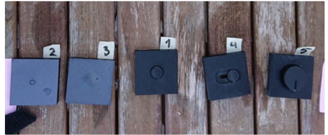
△ ILL. 95 Five different buttons were tested. From the left: flat button with rubber on top (2), convex button with rubber on top (3), a regular push button (1), the sliding button (4) and the turning dial button.
