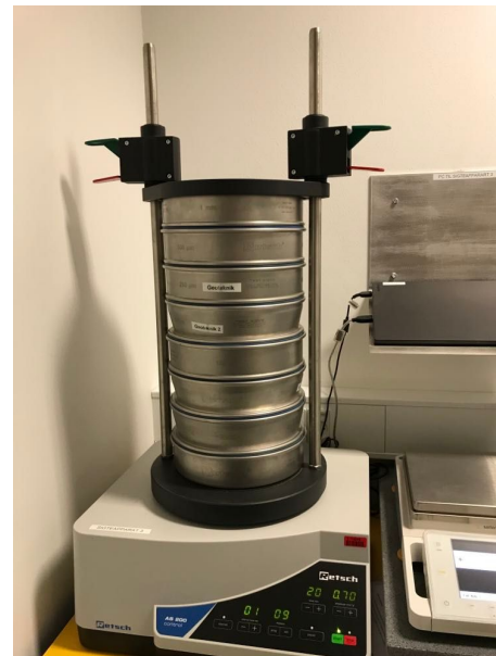
Figure A.1. Grain size distribution done in a sieving tower.
