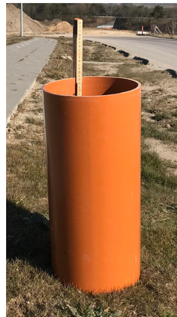
Figure B.1. Setup of the single ring infiltrometer. Ruler attached to the inner side of the pipe. Insertion depth kept at 5cm into the topsoil.
