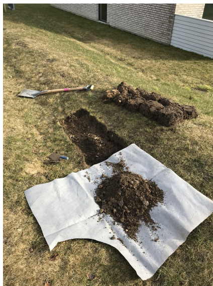
Figure A.2. Collection of loose soil samples from Marshalls Allé for further laboratory analysis.
