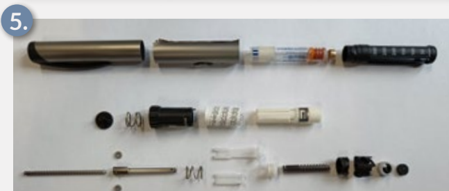
ILL. 42 exploded view of pens and pumps (App 3.5 + 3.12)
