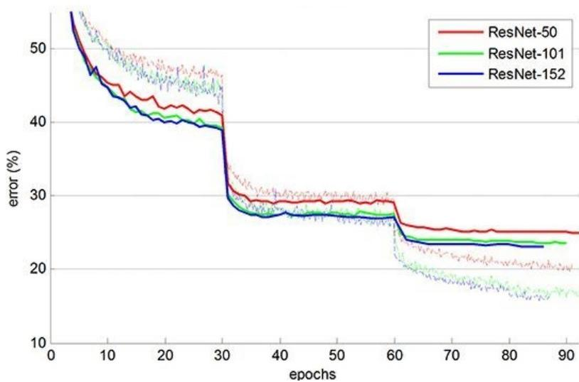
Figure 11: Error% decreases with addition of more layers (Resnet 50,101,152) [33]
