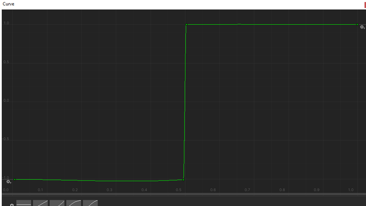
Figure 5.6: The Manipulation curve, the horizontal axis - time (0 to duration of the condition, mapped 0 to 1), and the vertical axis, representing what the value should be, in accordance to time.
