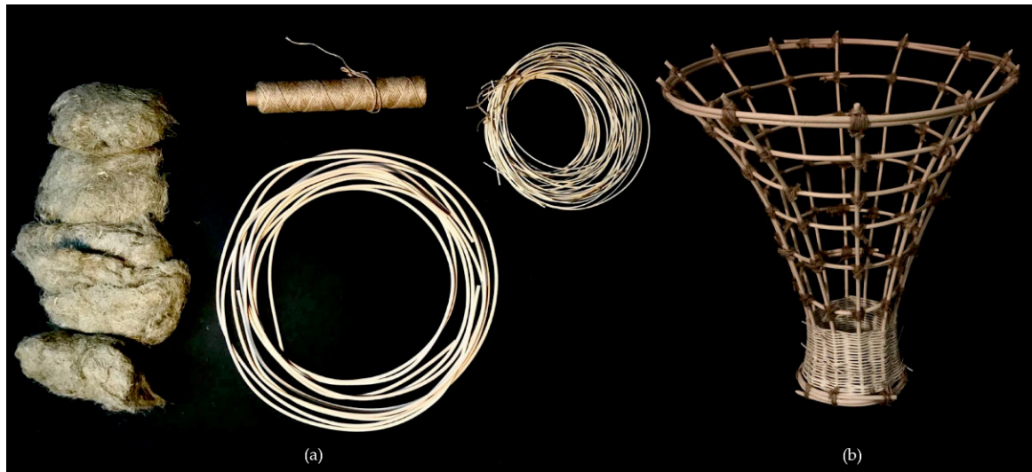
Figure 11. Material overview: (a) hemp fibers, rattan rods, jute fabric, (b) assembled rattan frame.
