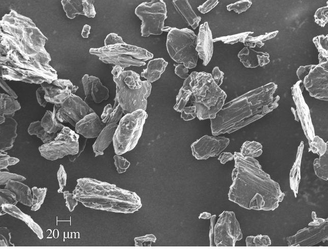
FIG. 1. Scanning electron microscopy image of the Timcal Timrex KS5-75TT graphite particles used in this study obtained using a Zeiss EVO LS15 with an EHT of 10kV.
