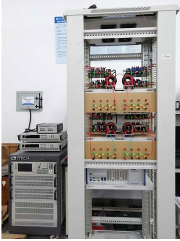
Fig. 6. A down-scaled laboratory prototype of MMC.
