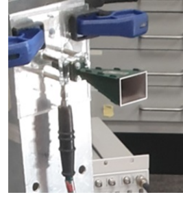
Fig. 2. Horn antenna as the receiver antenna in mechanical beam-steering experiment.
