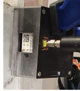
Fig. 3. 4 x 4 phased array antenna as the receiver antenna in electronic beam-steering experiment.
