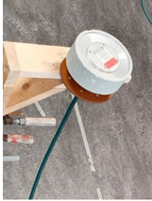
Fig. 1. Omnidirectional antenna as the transmitter antenna in both experiments.
