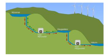
Fig. 3.19: Schematic of the planned pumped storage system [123].
