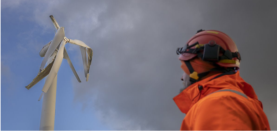
Fig. 1.7: The Nordtank wind turbine struck by lightening. Photo by B. Á. Rubeksen.
