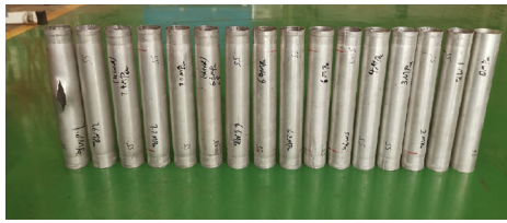
Fig. 9 Tubular specimens before and after hydraulic test.
