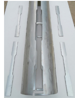
Fig. 6 Specimens for tensile test cut from tube along longitudinal direction.
