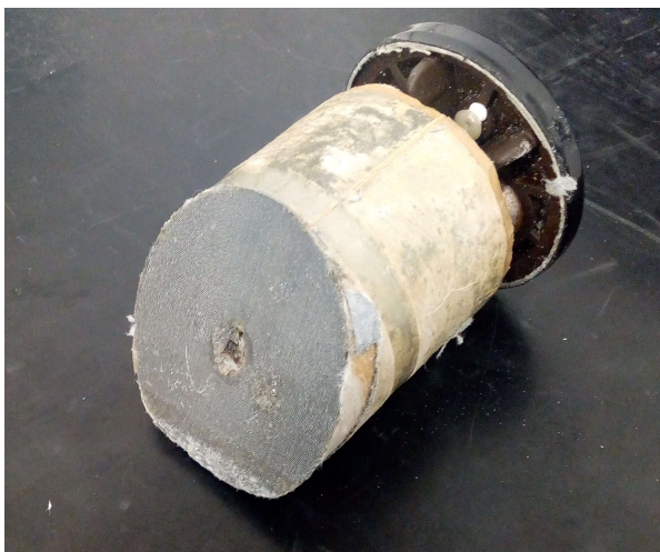
Fig. 8: Capacitor cut in half for measuring purposes.
