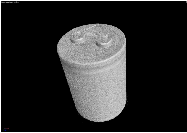
Fig. 7: 3D image obtained from the CT scan of the capacitor.
