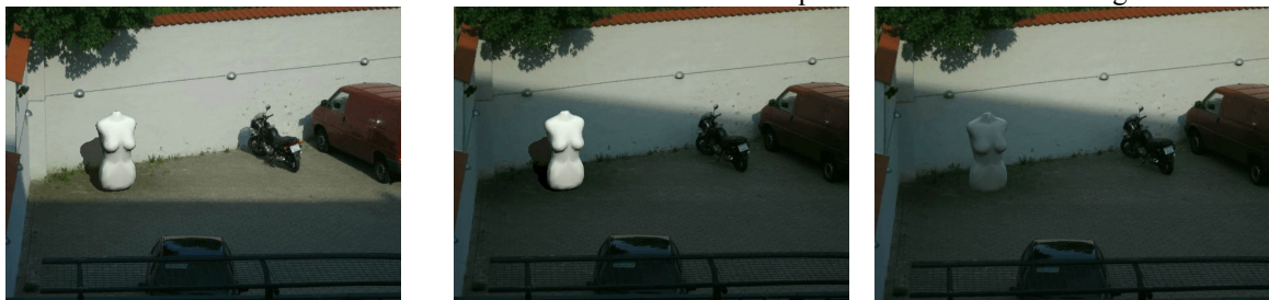
Figure 1: (Left) Virtual object augmented into a scene, calibrated to fit lighting of scene. (Middle) Scene-lighting changes, virtual object keeps previous shading, and stands out. (Right) Lighting of object is dynamically updated to fit the lighting of the rest of the scene.
