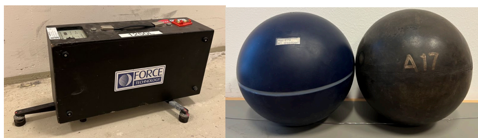
Figure 2 – Left: Tapping Machine B&K 3207; Middle: Impact Ball Nor279; Right: Impact Ball (Old Ball)
