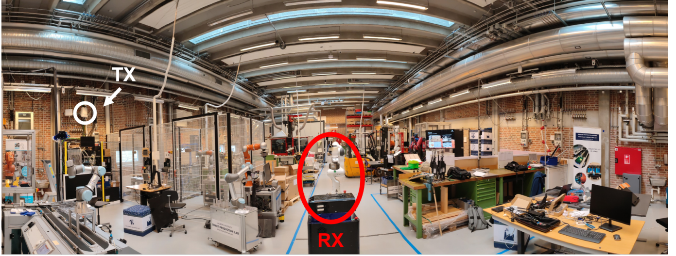
Fig. 1. View of the AAU 5G Smart Production Lab. The transmitter module (TX) is located on the left side. The scanner and the receiver antenna (RX) are located on the AMR system.
