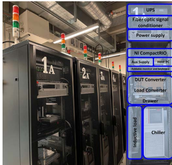
(b) Left: 6-unit, 19" industrial rack array; right: detailed configuration of one rack. Fig. 2. DC- and AC Power cycling test setup.
