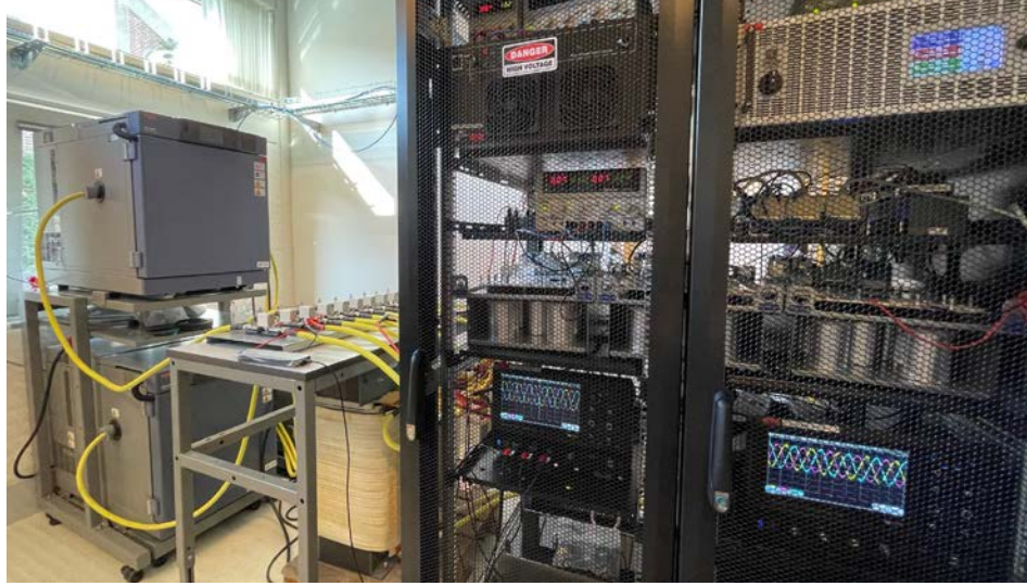
(b) Photo of the developed capacitor testing system.
