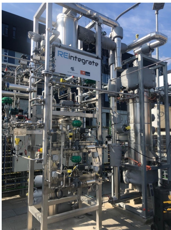
Figure 8: The first e-methanol pilot plant in Denmark (~ 220 ton/year) at Aalborg University (Power2Met, EUDP project).
