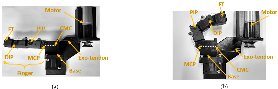
Figure 5. Artificial finger in its initial position for assessing (a) flexion and (b) extension. Note: the exotendons are not under tension since the artificial finger is in a relaxed state.
