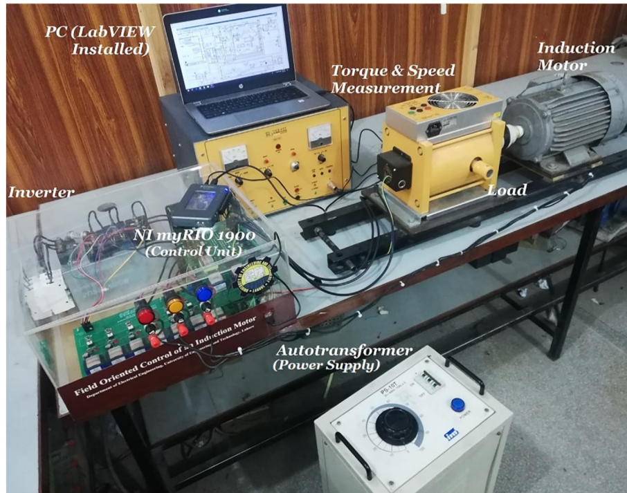
FIGURE 4 Induction machine drive testbed set-up
