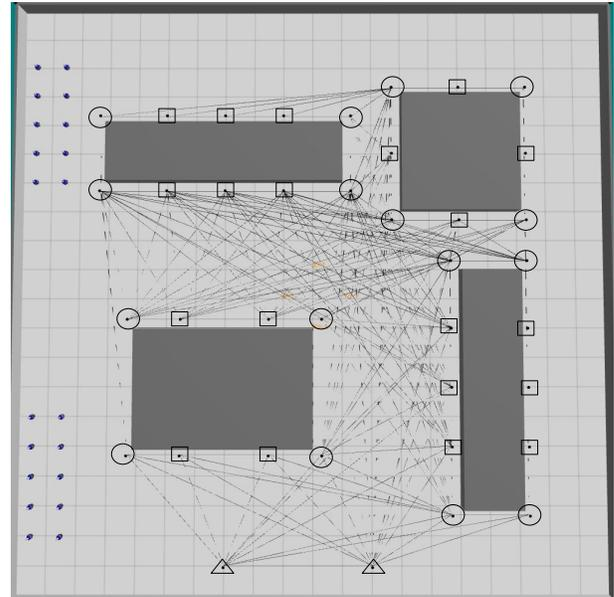
Figure 6: Factory map used in the experiments, containing four static obstacles, 20 workstations ( $\square$ ), 16 waypoints ( $\circ$ ), and two drop-off stations ( $\triangle$ ). 20 AMRs are placed in two groups to the left.
