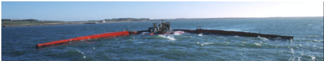
Figure 6: Wave Dragon prototype. Approaching waves are concentrated by the reflector towards the ramp.
