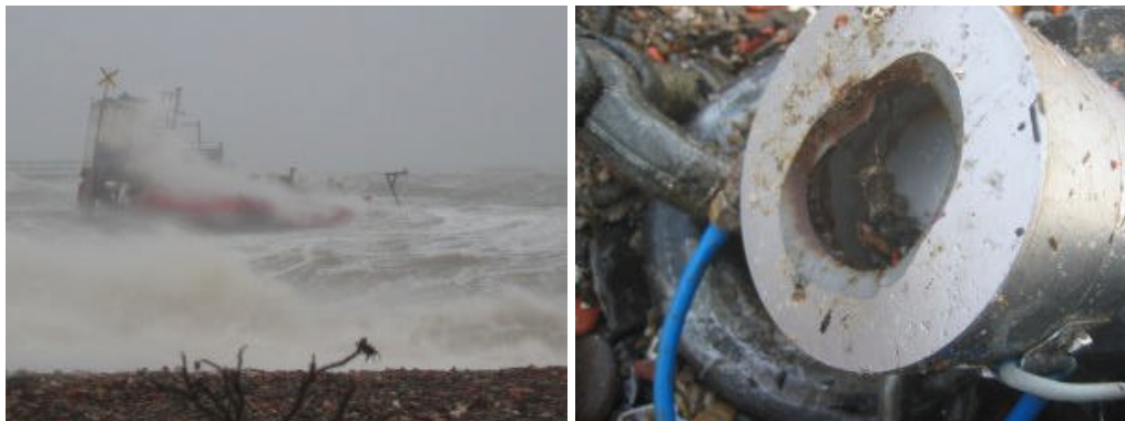
Figure 13: The WD stranded at the beach (left) after failure of the force transducer in the main mooring line (right).
