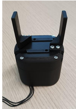
Fig. 1. First prototype of the 2-finger parallel gripper.
