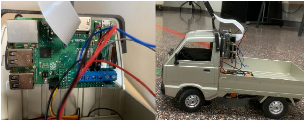
Fig. 1. Van vehicle adapted with Raspberry Pi 3 B+.
