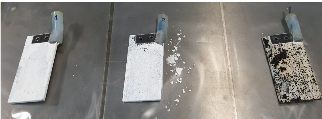
Figure 25. Triplets, blanks – cathodes after test and drying to 50°C
