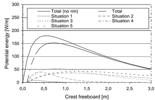
**Figure 7: Potential energy obtained in the basin per time and width unit as a function of the crest freeboard. Curves are calculated using the data from the 5 wave situations (after focusing by the wave reflectors) weighed with the time of occurrence. “Total” is the sum of the 5 situations, while “Total (no rim)” curve is the energy calculated with rim height  $r = 0$ .**
