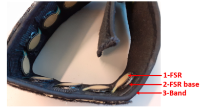
Fig. 2. Mounting of FSR sensor on the sensor band.
