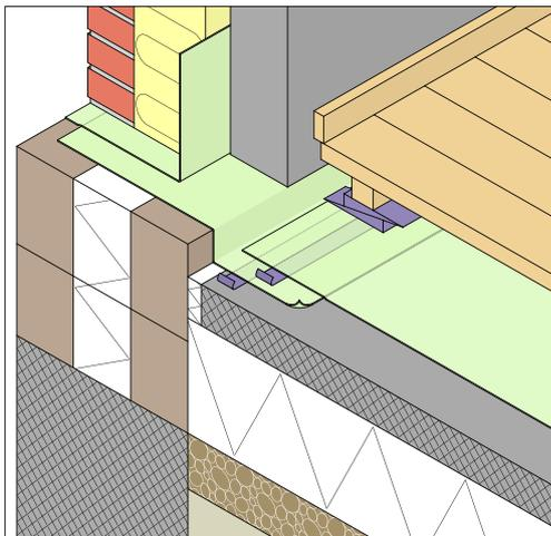
*Figure 3. The membrane is extended to the façade and is glued to the foundation, if necessary. The membrane is joined with the membrane laid out on the concrete slab and is protection both against moisture and radon. The membranes should be joined on a steady surface unless something else is recommended by the producer. The joints should be glued meticulously and the membranes should have a generous overlap, 100-150 mm. The joint should fix the overlap, be even and glued to the concrete slab.*
