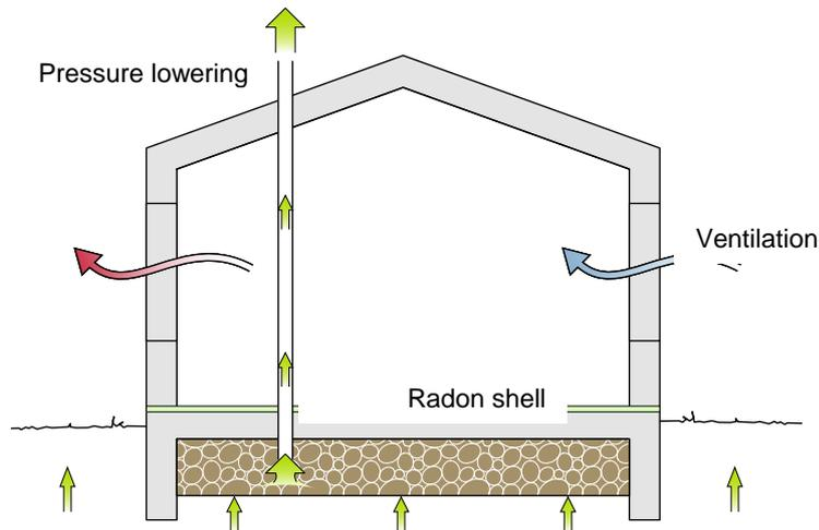
Figure 1. By combining three initiatives the radon penetration and concentration indoors can be controlled. 1) Establishing a shield that prevents radon from penetrating into the building. 2) Lowering the pressure difference over the building envelope facing the ground. 3) Diluting the indoor air in the building with outdoor air.
