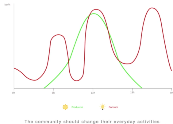
Figure 1: Conceptualising and explaining the concept of aligning energy activities after patterns of consumption and production within the energy community [12]
