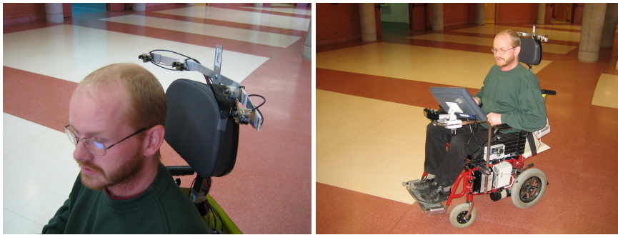
Figure 5. The sensors attached to the head rest piece of the SIAMO wheelchair.
