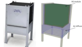
Figure 5. Real and virtual representation MBR module.
