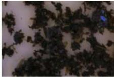
**Figure 1.** Flocculated manure. Irregular water-containing flocs (0.1 - 5 mm) formed during flocculation
