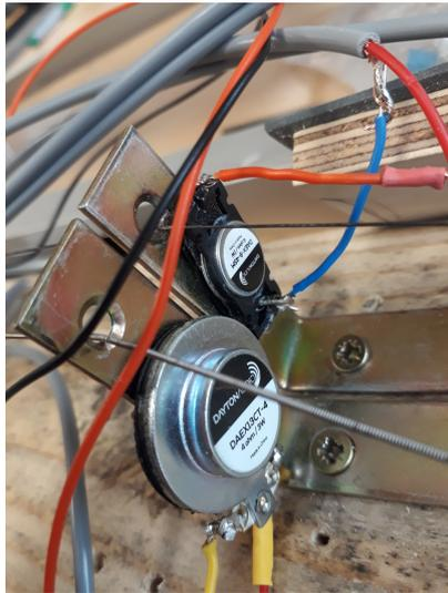
**Figure A.4:** Two transducers of different power assembled to the metal string holder (bridge) on the prototype
