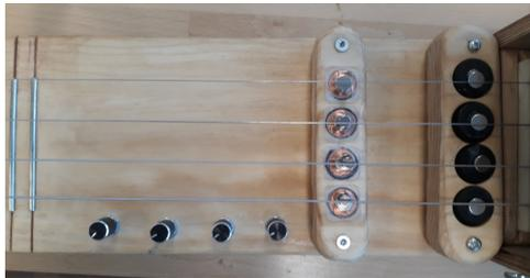
**Figure 4.3:** Detail view of the coils and potentiometers of the EBow Circuit
