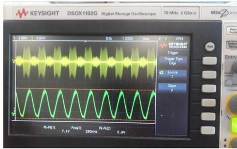
**Figure 2.5:** Example 3 of signal input and output forms as a result of testing different components in the circuit. The waveform of the output coil (green) resembles a sine wave oscillation
