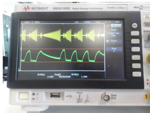
**Figure 2.4:** Example 2 of signal input and output forms as a result of testing different components in the circuit. The waveform of the output coil (green) shows a shark fin like or saw tooth form
