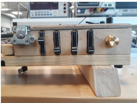
**Figure 4.6:** Detail view of the technology box with 4 faders and a potentiometer
