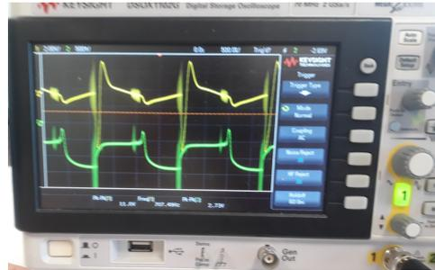
**Figure 2.3:** Example 1 of signal input and output forms as a result of testing different components in the circuit. The waveform of the output coil (green) shows a plateau form and spikes
