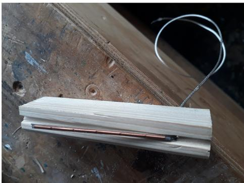
**Figure 4.2:** Disassembled Piezo PickUp as part of the Bridge
