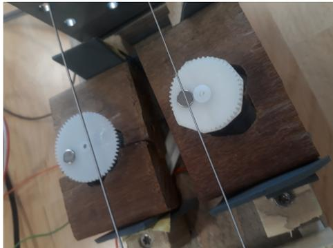
**Figure A.3:** Top view of two rotary motor with plastic capes and a magnet installed underneath the string of the prototype
