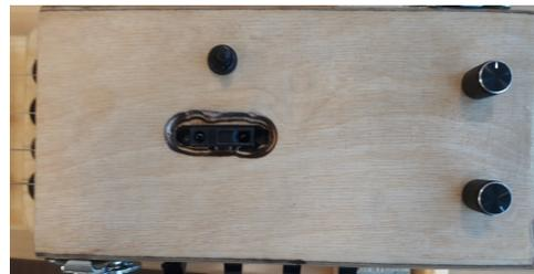
**Figure 4.5:** Detail view of the technology box with Infrared sensor, switch control and two potentiometers
