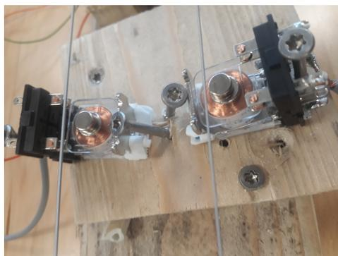
**Figure A.1:** Dismantled 12V DC Relay Coils for single string pickup
