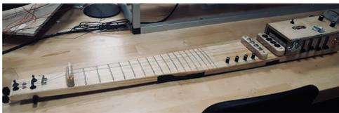
**Figure 4.1:** Final wooden Hardware Board with Frets, Strings, Coils and TechnicBox
