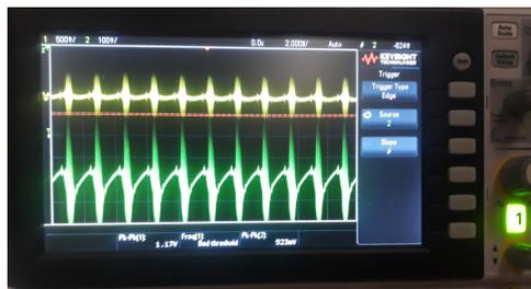
**Figure 2.6:** Example 4 of signal input and output forms as a result of testing different components in the circuit. Here the waveform looks like a shark fin with high spikes
