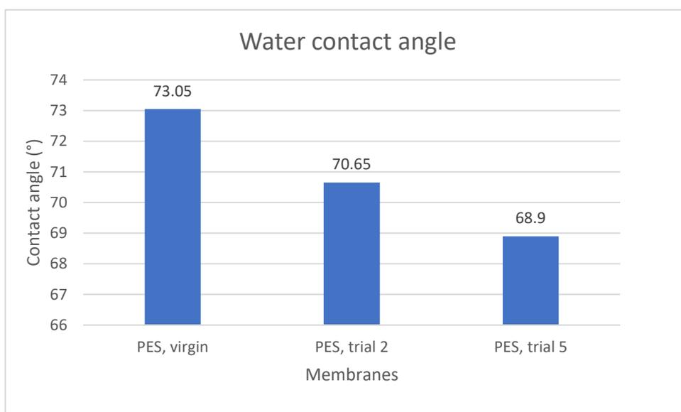
Figure 18) Water contact angle comparison for virgin, Trial 2 and trial 5 PES membranes
