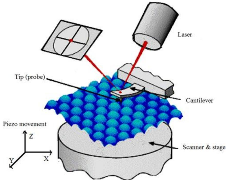
Figure 20) Schematic representation of an atomic force microscope[17]
