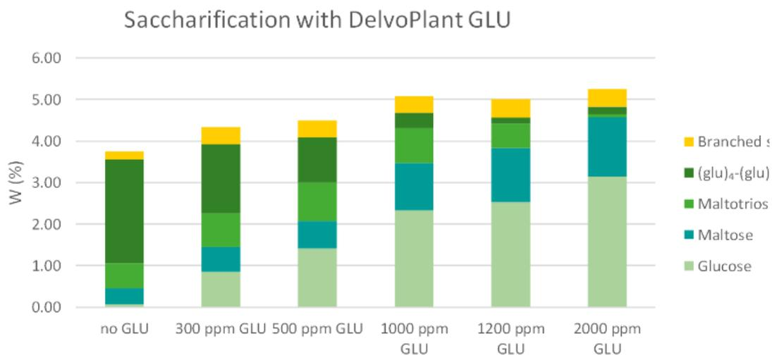
Figure 16) Effect on beta-glucosidase (GLU) concentrations on the formation of monomeric sugars in saccharification of oat slurry
