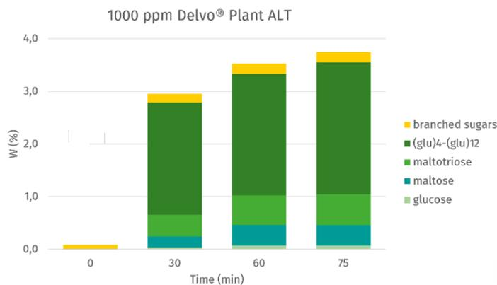
Figure 15) sugar content of liquefied oat slurry with alpha-amylase (Delvo Plant ALT)
