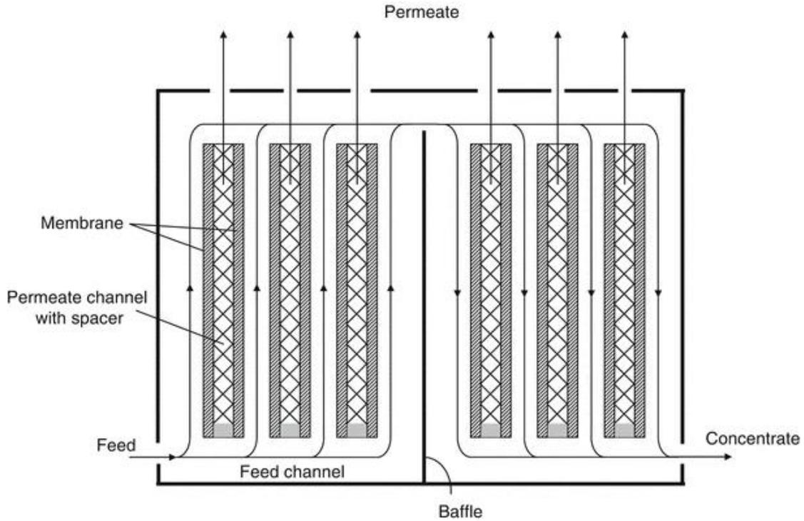
Figure 9: flow path for a plate-and-frame membrane module
