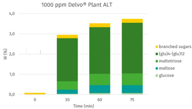
Figure 3) Liquefaction of oat slurry[12]
