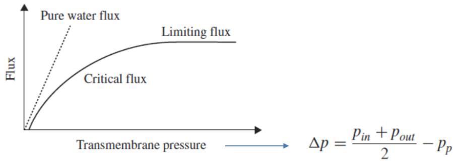
Figure 10) TMP vs flux curve.[24]
