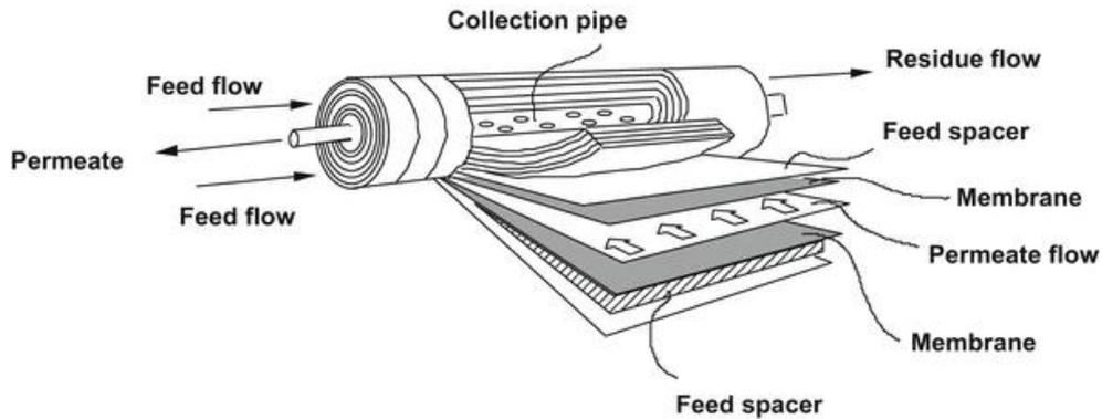
Figure 6: Schematic drawing of a spiral-wound module membrane and its components[20]
