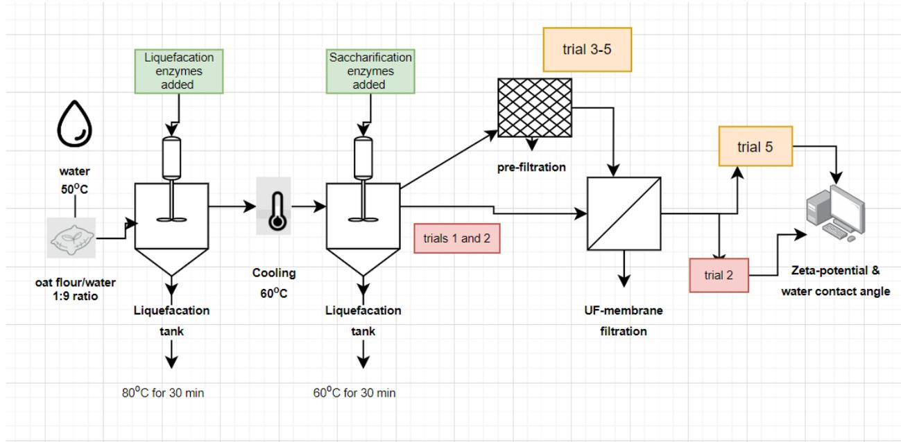
Figure 12: Flowchart over the whole process. the green boxes indicates the liquefaction and saccharification steps. The pink Boxes indicate the trials without pre-filtration and the orange boxes indicate the trials that underwent pre-filtration.
