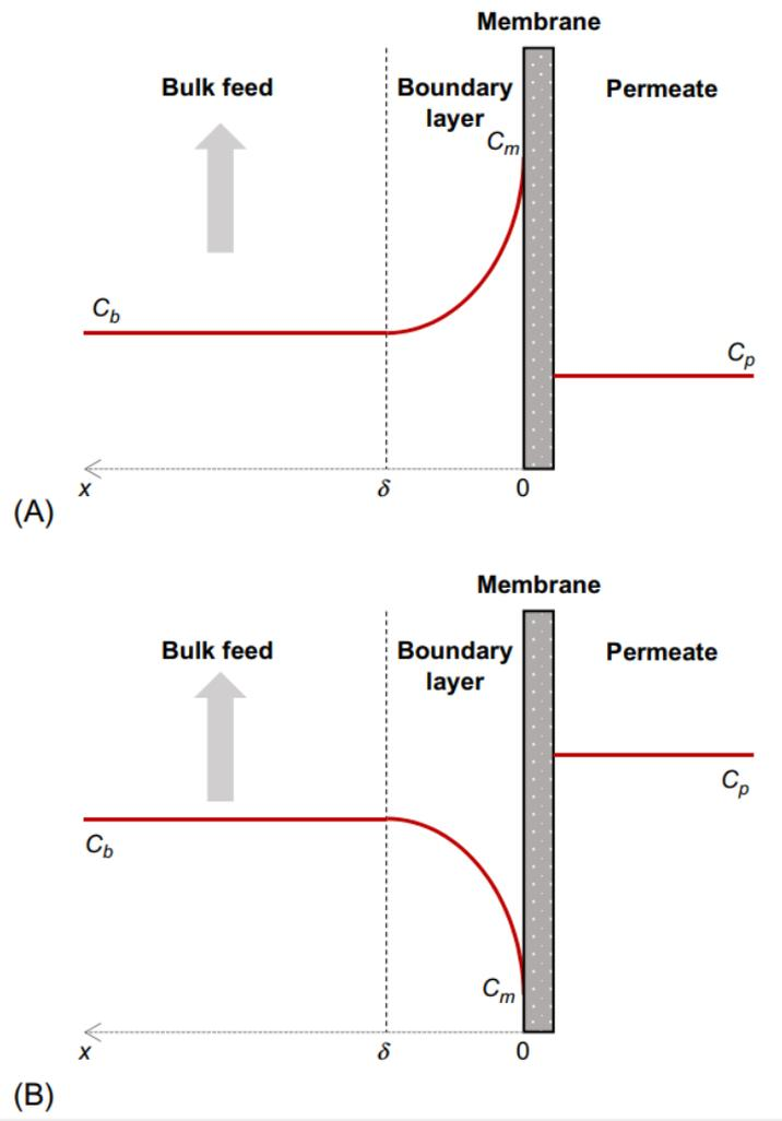
Figure 11) Concentration profile with concentration polarization: (A) mass transfer limited by the membrane and (B) mass transfer limited by the boundary layer.[10]
