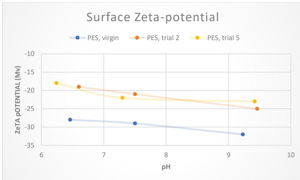
Figure 19) Membrane surface zeta-potential for virgin, trial 2 and trial 5 PES membranes
