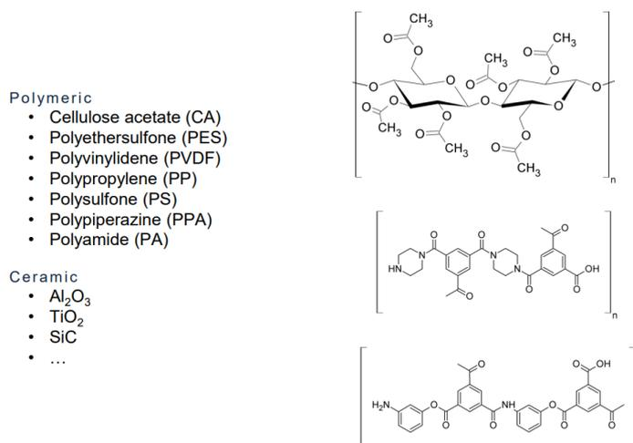
Figure 5) The two broad categories of membrane materials; polymeric and ceramic and their types[17]
