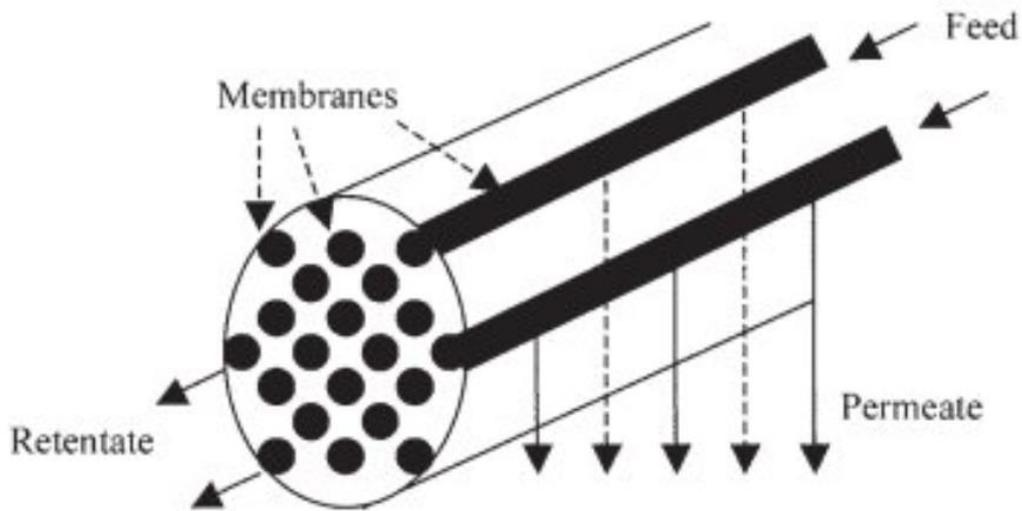
Figure 7) schematic drawing of a tubular membrane module
