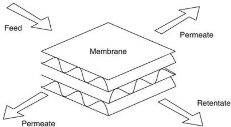
Figure 8: Schematic representation of a plate-and-frame membrane module
