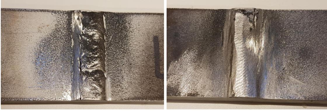
(a) Partial grinding of S690 specimen.
