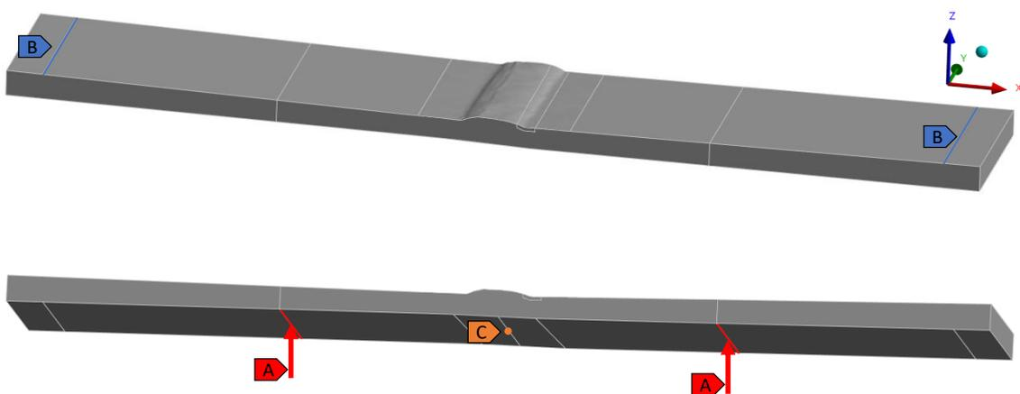
**Figure 5.1.** Boundary condition and load for FE model.
