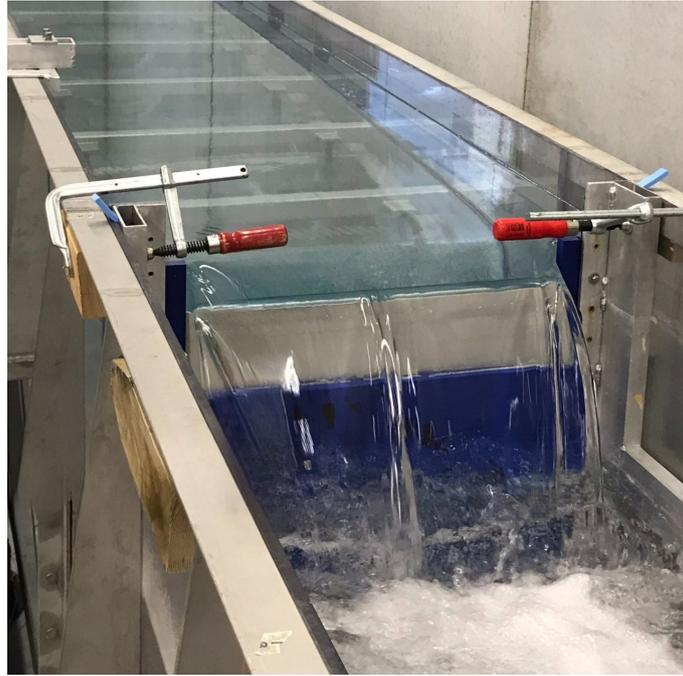
*Figure 4.2.* A photo of the weir placed in the channel.
